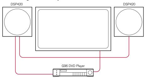
The DSP420 can be connected directly to almost any source that provides a PCM SPDIF output, including CD or DVD players, some PC soundcards, and digital satellite decoders.
