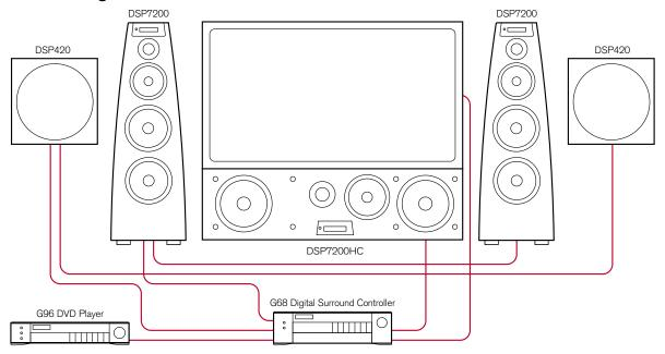
DSP420 loudspeakers can be used in conjunction with a Meridian Surround Processor to provide the two rear channels, and optionally two additional side channels, to create an unobtrusive surround system with superb music and cinema sound.
